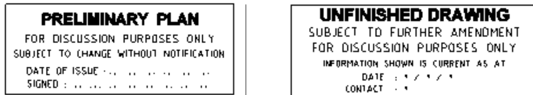
Figure 1.1: Preliminary or Unfinished Drawing Labels
